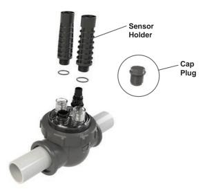
Figure 17. Sensor Holder Installation
