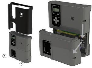
Figure 8. Remove Controller Lower Cover
