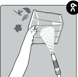
Clean the filter basket with a hose.
